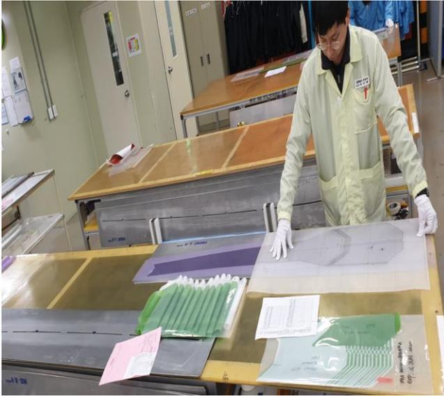
737 MAX SPAR CHANNEL MYLAR INSPECTION
