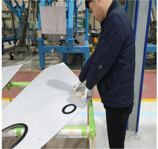
PAINT WET ADHESION INSPECTION
