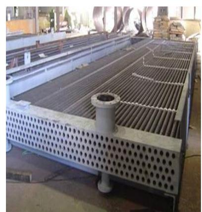
Air Cooled Heat Exchanger
