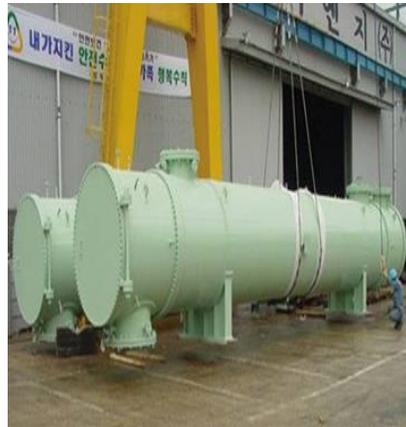
CCW(Closed Cooling Water) Heat Exchanger
